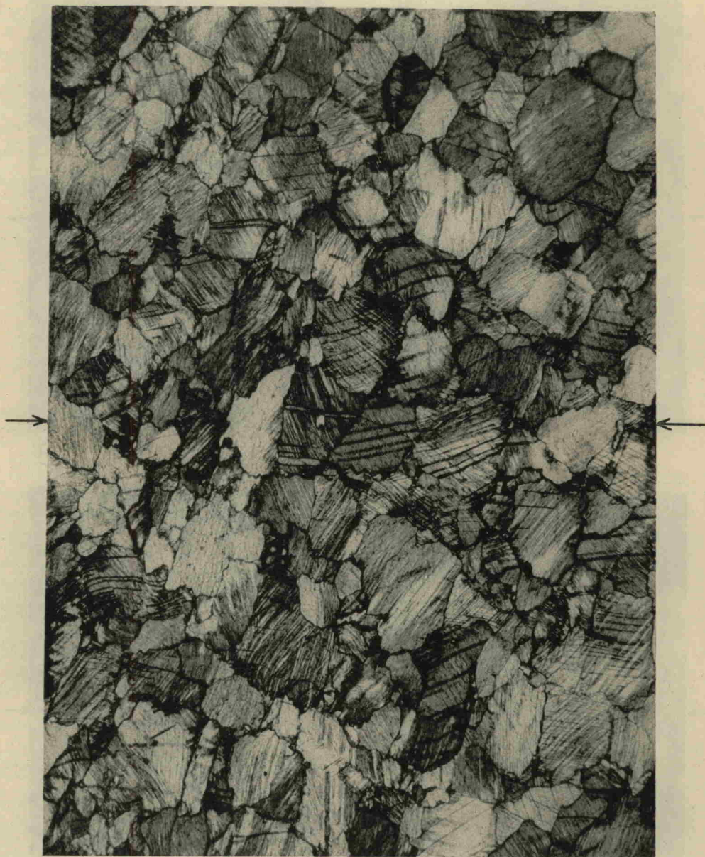
PHOTOMICROGRAPH OF DEFORMED YULE MARBLE
